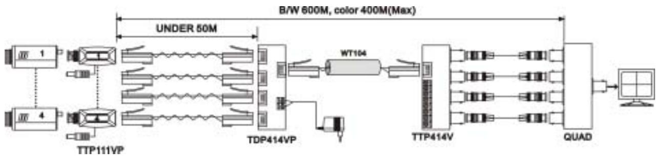
**Note:** Camera power send from TDP414VP cable hub station (50meters), work with TTP111VP. TDP414VP including " regulated power adapter" must work with "non-regulated camera". Once your camera built in regulated IC, the adapter must alternate to NON-Regulated.
